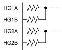
Figure 29. HG Double Power Connection
