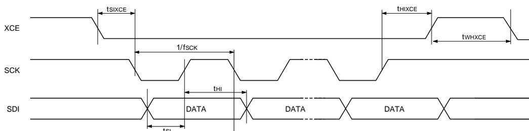
Serial Control Interface Timing (Sub-LVDS)
