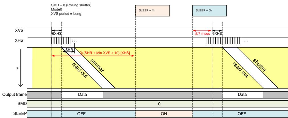
Low Power Consumption Drive in Integration Time When Using Rolling Shutter Operation (Sub-LVDS)
