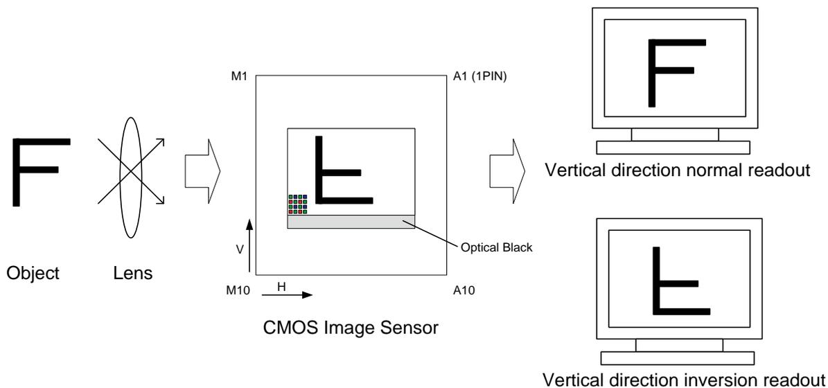
Note) Arrows in the figure indicate scanning direction during normal readout in the vertical direction.
