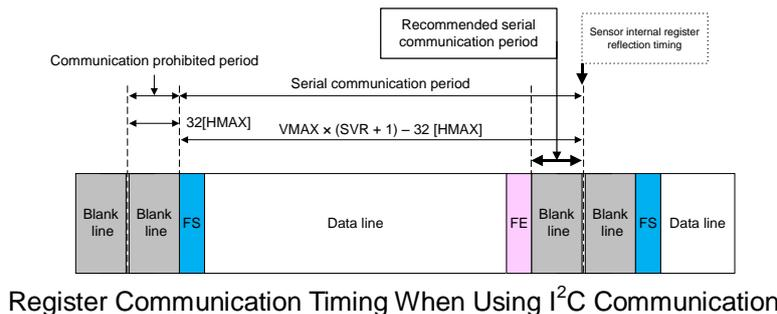
Register Communication Timing When Using I<sup>2</sup>C Communication
