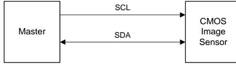
Pin connection of serial communication
